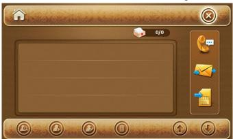
Send SMS: select one connector in the list and click this button to send SMS.
