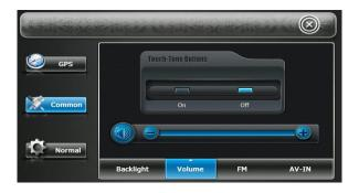
Click the icon volume in the setup interface to log into the interface of Volume Adjustment as
