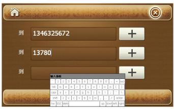
Input the phone number to the entry box directly, or click the icon 🕇 to log into the phone book to select the disired connector to add the number( if need to send SMS to multi person, you can continue to input the number to the entry box).
